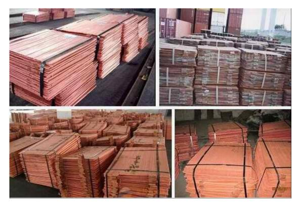
It refers to the crude copper (copper content of 99%) made of thick plate as anode, pure copper made of thin sheet as cathode, with sulfuric acid (H2SO4) and copper sulfate (CuSO4) mixed liquid as electrolyte. After electrifying, copper dissolves into copper ions (Cu) from the anode and moves to the cathode. After reaching the cathode, it will obtain electrons and precipitate pure copper in the cathode, which is of high quality and can be used to make electrical products.
